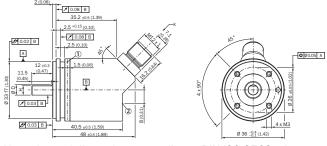
Non-tolerated dimensions according to DIN-ISO 2768-mk
