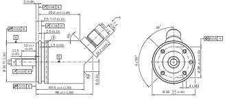
Non-tolerated dimensions according to DIN-ISO 2768-mk
