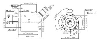
Non-tolerated dimensions according to DIN-ISO 2768-mk
