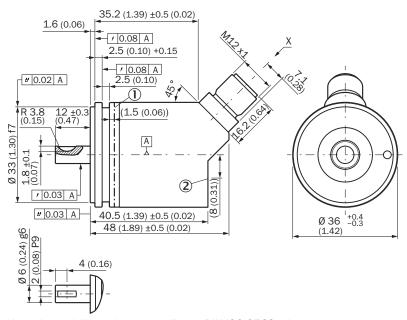
Non-tolerated dimensions according to DIN-ISO 2768-mk
