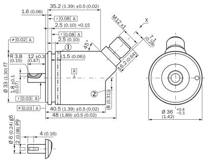
Non-tolerated dimensions according to DIN-ISO 2768-mk
