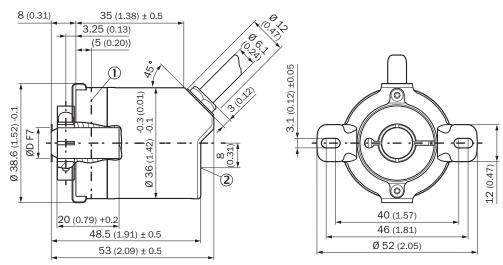
Measuring point for operating temperature
