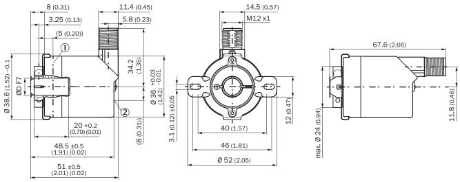
① Measuring point for operating temperature
