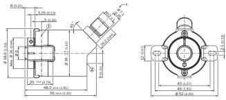
Non-tolerated dimensions according to DIN-ISO 2768-mk
