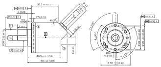
Non-tolerated dimensions according to DIN-ISO 2768-mk
