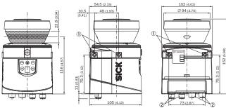
① Mounting hole M5 x 7.5 ② Connector M12
