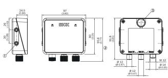
Structure and device dimensions, unit: mm (inch), decimal separator: period
