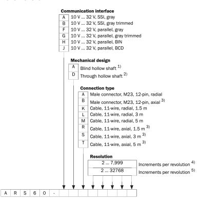
$<sup>^{1)}</sup>$  Communication interface J: Increments per revolution 2  $\dots$  7999 possible.
