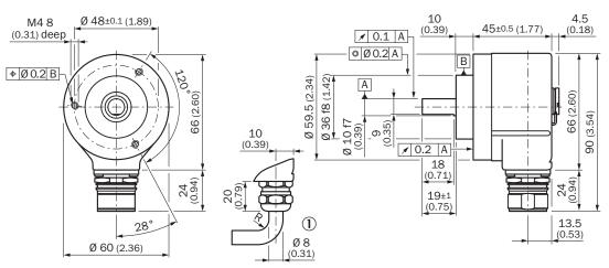
General tolerances according to DIN ISO 2768-mk ① R = min. bending radius 40 mm
