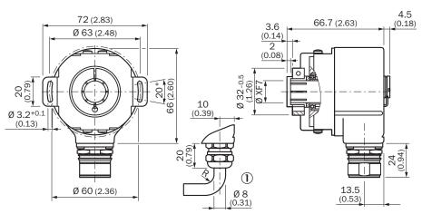
General tolerances according to DIN ISO 2768-mk ① R = min. bending radius 40 mm
