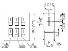
3 pairs included with apertures A, B, C. Self-adhesive backing for easy mounting. Apply stick-on mask to WS100 and WE100 front lens. For small object detection or increasing
