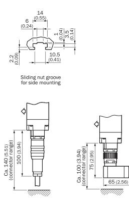
Cable sockets M26 x 11 + FE with crimp contacts
