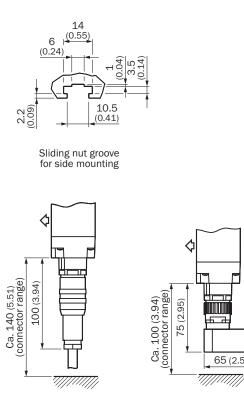
Cable sockets M26 x 11 + FE with crimp contacts
