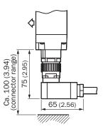
Cable sockets M26 x 11 + FE with crimp contacts
