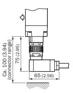
Cable sockets M26 x 11 + FE with crimp contacts
