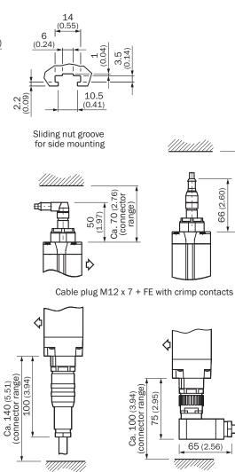
Cable sockets M26 x 11 + FE with crimp contacts
