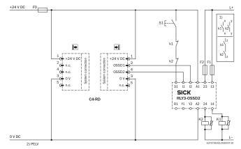
① Output circuits: These contacts must be incorporated into the control such that the dangerous state is brought to an end if the output circuit is open. For categories 4 and 3, they must be incorporated on dual-channels (x, y paths). Single-channel incorporation into the control (z path) is only possible with a single-channel control and taking the risk analysis into account.
