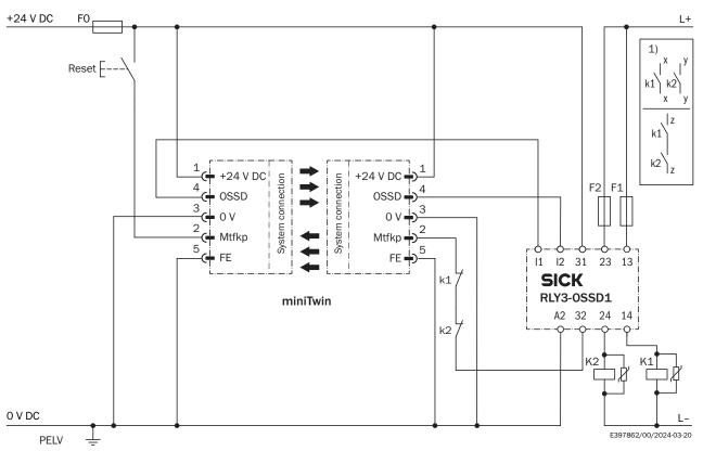
miniTwin safety light curtain to RLY3-OSSD1 safety relay with restart interlock and external device monitoring
