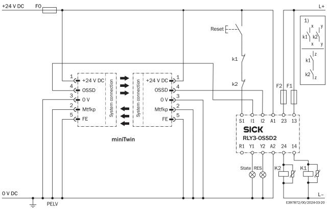
① Output circuits: These contacts must be incorporated into the control such that the dangerous state is brought to an end if the output circuit is open. For categories 4 and 3, they must be incorporated on dual-channels (x, y paths). Single-channel incorporation into the control (z path) is only possible with a single-channel control and taking the risk analysis into account.
