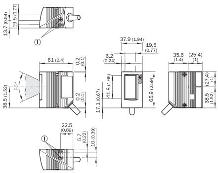
① Blind hole thread M5, 5 mm deep (2 x), for mounting
