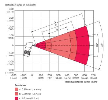
① Diagram applies to focus position of 280 mm
