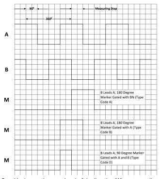
$\mbox{\sc Cw}$  with view on the encoder shaft in direction "A", compare dimensional drawing.
