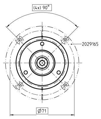
Mounting requirements for small servo clamp
