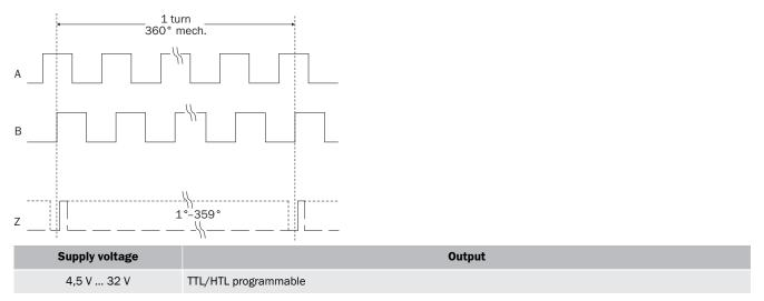
Electrical zero pulse width can be configured to 90°, 180°, or 270°. Width of the zero pulse in relation to a pulse period.
