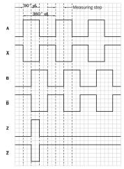
CW with view on the encoder shaft in direction "A", compare dimensional drawing. Maximum revolution range
