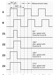
$\mbox{\sc Cw}$  with view on the encoder shaft in direction "A", compare dimensional drawing.
