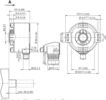
$\bigcirc$  Cable diameter = 5.6 mm +/- 0.2 mm bend radius = 30 mm
