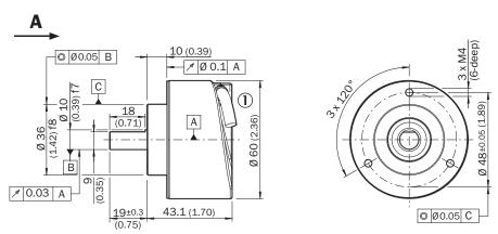
① Cable diameter = 5.6 mm + /-0.2 mm bend radius = 30 mm
