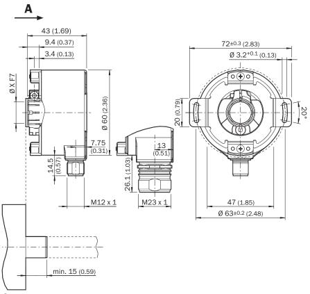
① Cable diameter = 5.6 mm + /-0.2 mm bend radius = 30 mm
