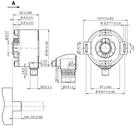
(1) Cable diameter = 5.6 mm +/- 0.2 mm bend radius = 30 mm
