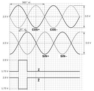
For clockwise shaft rotation, looking in direction "A" (see dimensional drawing)
