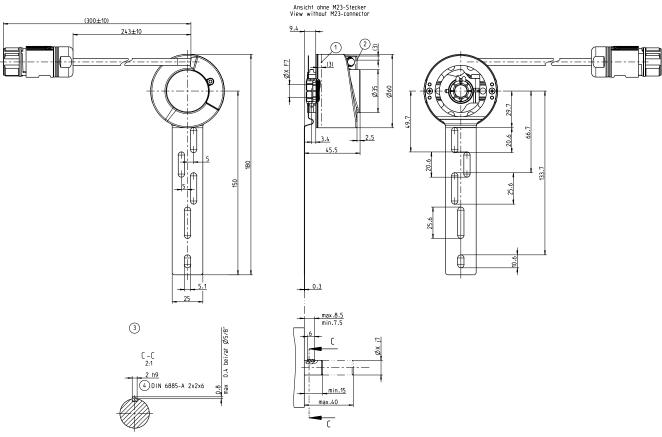
① Operating temperature measuring point (freely selectable, in each case circumferential at the housing surface, approx. 3 mm from the flange)
