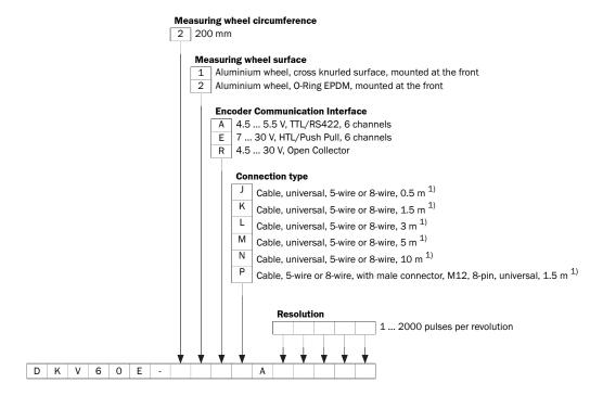
$<sup>^{1)}</sup>$  The universal cable outlet is positioned so that a kink-free cable in a radial or axial direction is possible.
