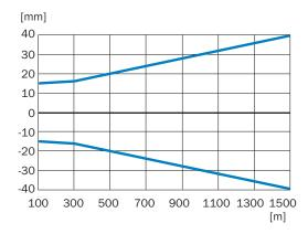
Typically DL1000, x-axis: Distance, y-axis: Typical measurement accuracy
