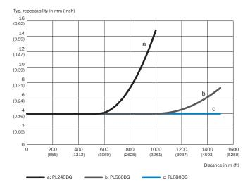
DL1000 for various reflector types, with 4 ms measurement cycle time
