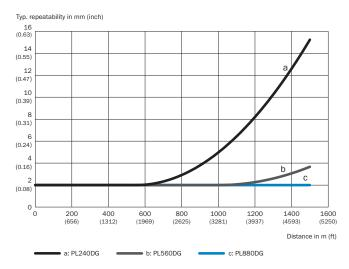
DL1000 for various reflector types, with 16 ms measurement cycle time
