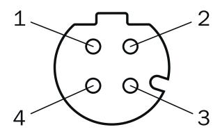
M12 female connector, 4-pin, D-coded
