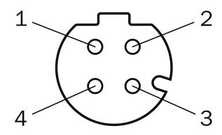
M12 female connector, 4-pin, D-coded
