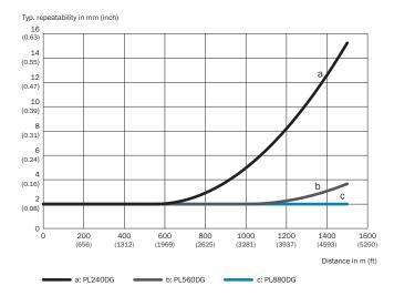
$\ensuremath{\mathsf{DL}} 1000$  for various reflector types, with 16 ms measurement cycle time
