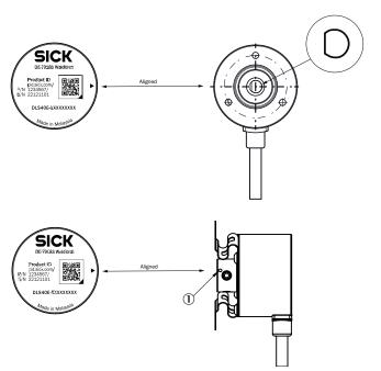
You can see the position with the mark on the rear side of the encoder 1 Zero pulse mark on housing
