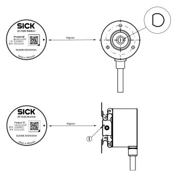
You can see the position with the mark on the rear side of the encoder  ${\tt \textcircled{1}}$  Zero pulse mark on housing
