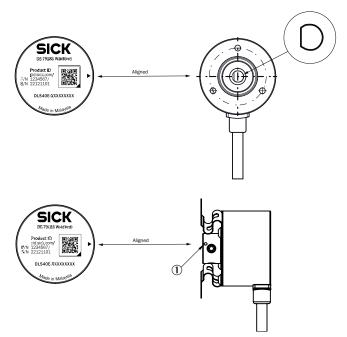
You can see the position with the mark on the rear side of the encoder Zero pulse mark on housing
