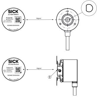
You can see the position with the mark on the rear side of the encoder 1 Zero pulse mark on housing
