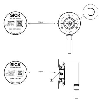
You can see the position with the mark on the rear side of the encoder  ${\tt \textcircled{1}}$  Zero pulse mark on housing
