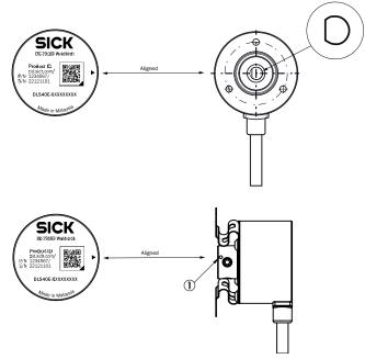
You can see the position with the mark on the rear side of the encoder Zero pulse mark on housing
