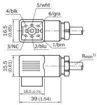
$\bigcirc$  Minimum bend radius at dynamic use R<sub>min</sub> = 20 x cable diameter
