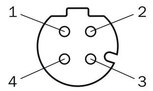
M12 female connector, 4-pin, D-coded
