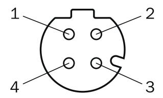
M12 female connector, 4-pin, D-coded
