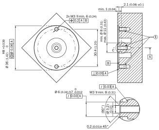
①  $3 \times M3$  drill holes, screw with hex key size, s = 2.5 mm
