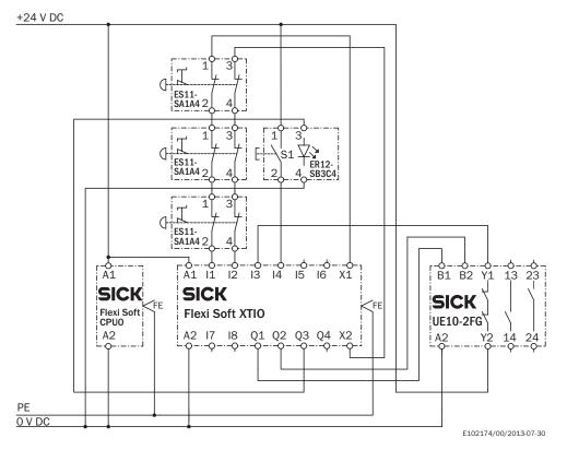
ER12 reset pushbutton and ES11 emergency stop pushbutton to UE43 safety relay
