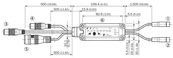
1 Port A, cable with female connector, M8, 4-pin
