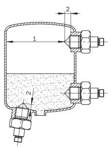
The apex should protrude into the container
